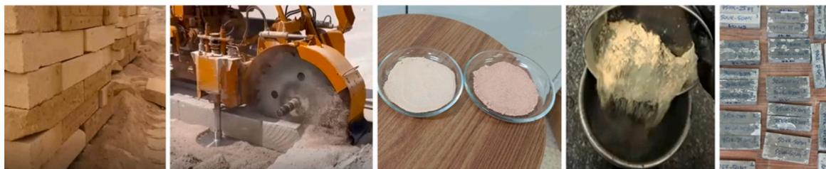
Fig. 1. Stone-cutting waste (SW) preparation process in factory and mortar production in the laboratory.
